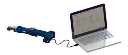
Start the SmartTool-Manager, log in and read out the current tool by clicking on "read". Now you can edit the settings as described in the following steps. So that the tool parametrization is not lost we recommend saving this separating under another name.
