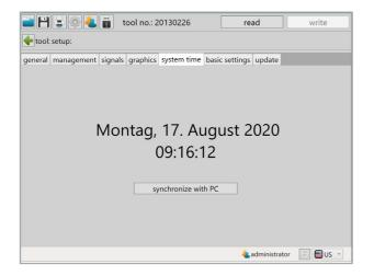
Under System time, the tool's Real Time Clock (RTC) can be synchronised with the time of the PC.
