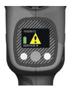
The service counters can be parametrised with the SmartTool-Manager under the "Service" user. The respective value entered will be multiplied by 1,000, i.e. when entering 10 the service notification will appear on the display after 10,000 sets. If you enter 0 the function is deactivated.
